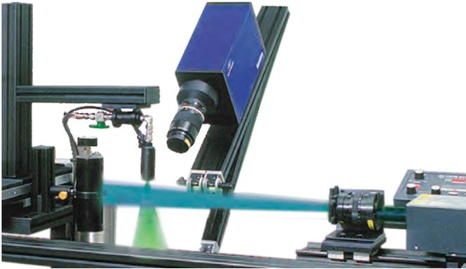
The Laser Induced Fluorescence (LIF) signal is proportional to the droplet mass and, therefore, contains a different information from what can be observed with purely Mie scattered light, which is proportional to the surface of the droplet. In combination with PIV the mass flux can be derived.
