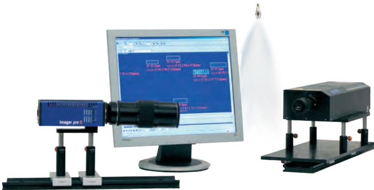
The approach with interferometric Mie Imaging (IMI) is recommendable for scarce sprays and uses a laser light sheet thus observing a larger area than Shadowgraphy. From defocused imaging in forward scattering direction interference fringe patterns are recorded which contain the information about droplet size in the fringe frequency.
