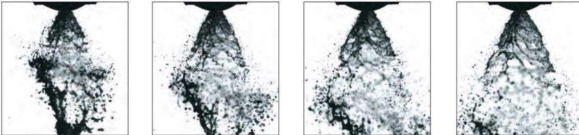
*Spray propagation: high-speed imaging at several kHz*
