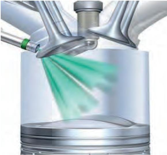
Nowadays laser imaging is a routinely used measurement tool for the investigation of fuel sprays in high pressure test cells or directly inside the combustion chamber. Keyhole imaging can be realized using laser and camera endoscopes, respectively.
