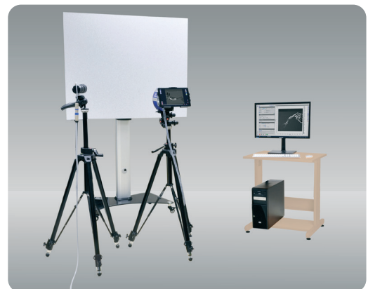
FlowBOS setup with pattern projected on a background surface
