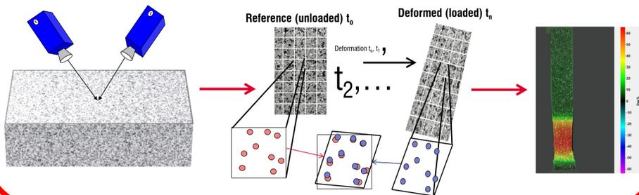
• Digital Volume Correlation (DVC) uses 3D volume images of materials created by X-Ray CT scanners, Magnetic Resonance Imaging (MRI), or any other system capable of generating volumetric images. The reconstructed volume images are then used to calculate displacements and strains that have occurred between a reference and some deformed state.
