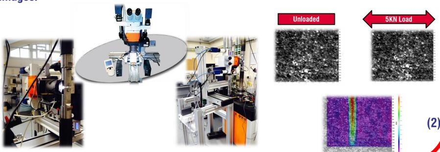
• A notch sample of nuclear graphite was scanned during loading. DVC was then used to identify displacements, strains and later a 3D crack opening displacement (COD). This study highlighted a high strain region ahead of the apparent location of the crack tip, designated as the 'Fracture Process Zone' where microcracks are shown as additional displacement regions.
