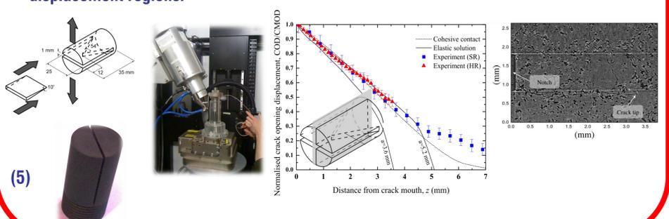
• Macro scale DIC was conducted on a concrete beam subjected to a three point bend loading process. Ultra high spatial resolution was achieved by using small subset sizes. Whilst small subsets have lower precision, they give higher spatial resolution, enabling the goal of accurate crack location detection. The highlighted red region shows areas where cracks would not normally be identifiable in the raw image but become obvious when studying the strain data
