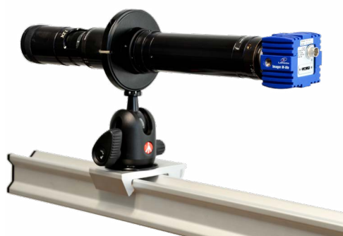
Zoom lens with M-lite camera mounted onto an X48 rail
