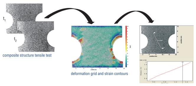
place virtual extensometer or strain gauge after the test
