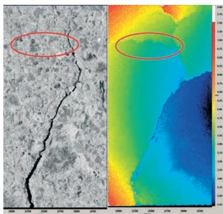
Because it is a full field technique and not restricted to obtaining data at the gauge location, **StrainMaster** can be used to identify strain hot spots, and subsequent crack initiation and propagation.
