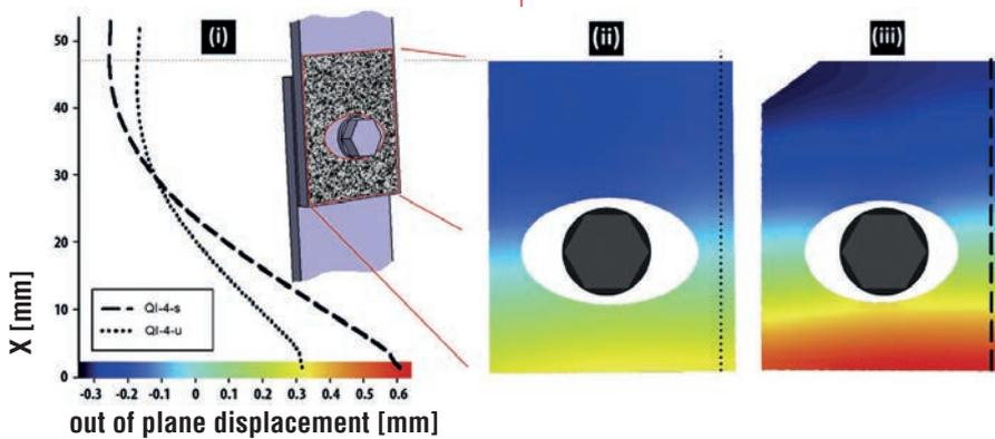
Composites represent another area where we are still trying to properly characterize the material for input into finite element models. **StrainMaster** has been used for various composite testing including pre-damaged panels, and compression after impact. In the left example two composite panels connected via a bolted joint have been studied using a **StrainMaster** system. The out of plane deformation is shown here.
