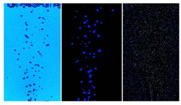
Phase separation in DaVis: both phases (left), bubble flow (middle) and liquid flow (right).
