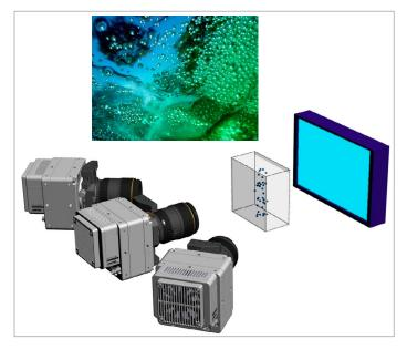
High-speed tomographic shadow imaging setup investigating multiphase flows in 3D.
