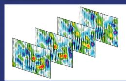
Spatial and temporal derivatives From one velocity field a range of spatial derivatives can be calculated such as vorticity and shear stress. Ensemble statistics provide additional information like turbulent kinetic energy or Reynolds stresses. Time-resolved velocity fields recorded with high-frame-rate cameras and high frequency laser allow for deeper dynamic insights about flow field evolution, fluid element trajectories, acceleration and turbulence statistics.
