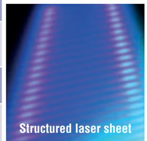
**Mie** Mie scattering is elastic light scattering caused by surface interaction. The wavelength is not changed. The signal strength is proportional to the surface area of the droplet.
