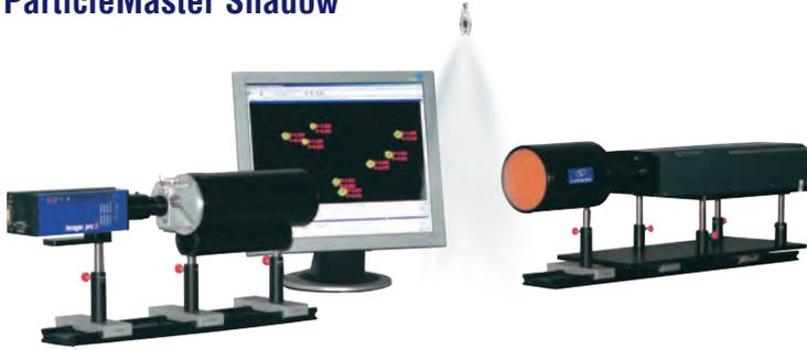
Based on imaging shadow projections of droplets the method of Shadowgraphy is applied in a small volume at a desired position within a spray (local). Quantitative absolute results are obtained and a range of light sources from pulsed LEDs to lasers can be used as backlight source. A long distance microscope assures a safe working distance at a high magnification to even detect very small droplets.
