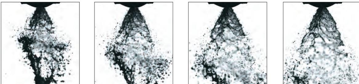
*Spray propagation: high-speed imaging at several kHz*
