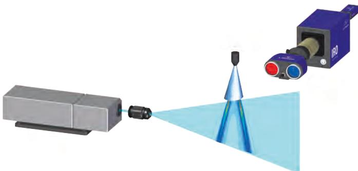
An instantaneous global droplet size map is obtained from the LIF/Mie technique where simultaneously a fluorescence signal (proportional to droplet volume) and a Mie signal (proportional to surface area) are recorded and divided by each other. This gives the Sauter Mean Diameter (SMD,  $D_{32}$ ) from a single laser pulse (fluorescent tracer required).
