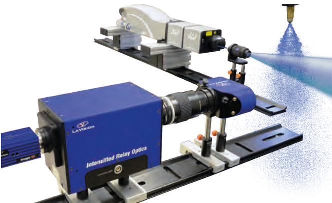
Laser Induced Exciplex Fluorescence (LIEF) allows simultaneous visualization of the two phases. Due to the special LIF tracers the signals from the liquid and the vapor phase can be spectrally separated by optical filters.
