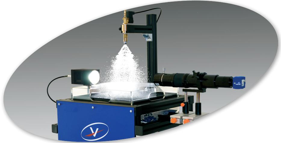
Cumulated statistics are size histograms, scatterplots and weighted averages, like Sauter Mean Diameter ( $D_{32}$ ), mean diameter ( $D_{10}$ ), volume percentiles (10, 50, 90%) and more.
