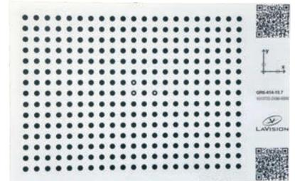
The calibration process enables the system to map from the camera space to the real world space. The calibration plate can be inside a chamber or within a liquid.
