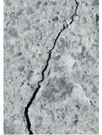
By following the surface pattern, local surface displacement can be calculated everywhere, and a whole field map of the displacement and strain can be calculated.
