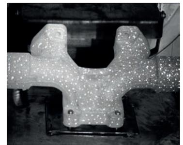
*DIC measurements of a hot (800°C) exhaust manifold - with filter (left) and without filter (right) Acknowledgement: images taken during a project with KTH Royal Institute of Technology (Sweden) and Scania.*
