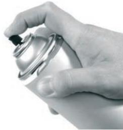
The optimum pattern for the technique is a random, rich in contrast, speckle pattern which is typically created with standard aerosol paints. In some cases the natural surface pattern may be suitable (e.g. concrete).
