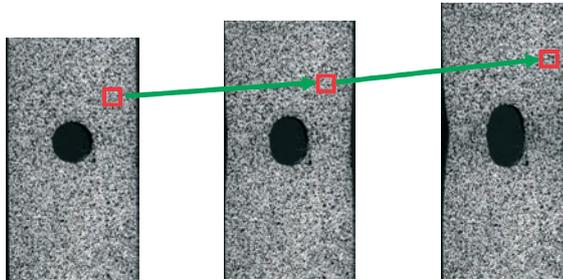
The pattern (which can be natural, or applied) is tracked all over the surface of the imaged material. By following the pattern everywhere the local displacement is calculated.
