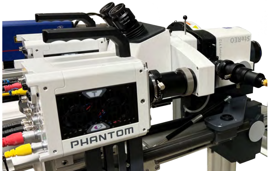
Stereo microscope based DIC system investigating fatigue crack growth
