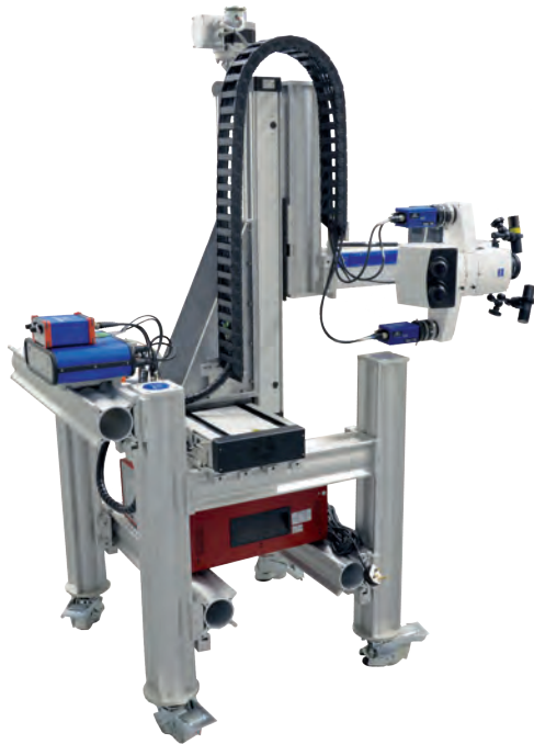
Complete micro-DIC system on moveable cradle
