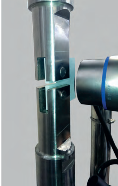
Stereo microscope based DIC system investigating fatigue crack growth
