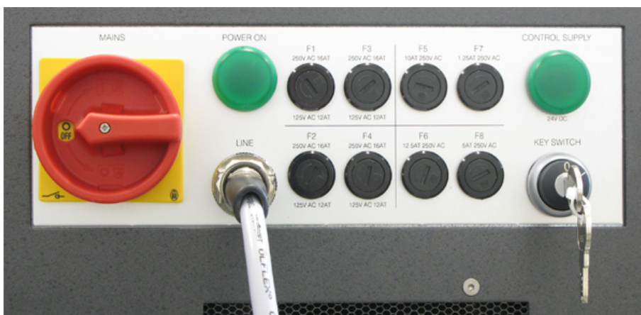
Figure 1.4: Controls at the rear of the laser housing; the mains switch is located on the left side, the key switch on the right
