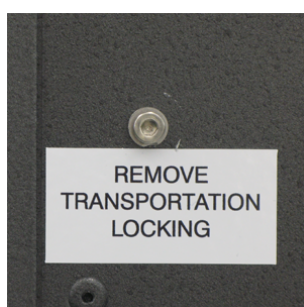
Figure 1.1: Transportation screw at the back of the laser housing; please remove before operating the laser
