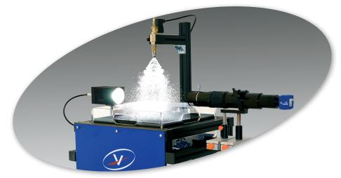
Cumulated statistics are size histograms, scatterplots and weighted averages, like Sauter Mean Diameter ( $D_{30}$ ), mean diameter ( $D_{10}$ ), volume percentiles (10, 50, 90%) and more.
